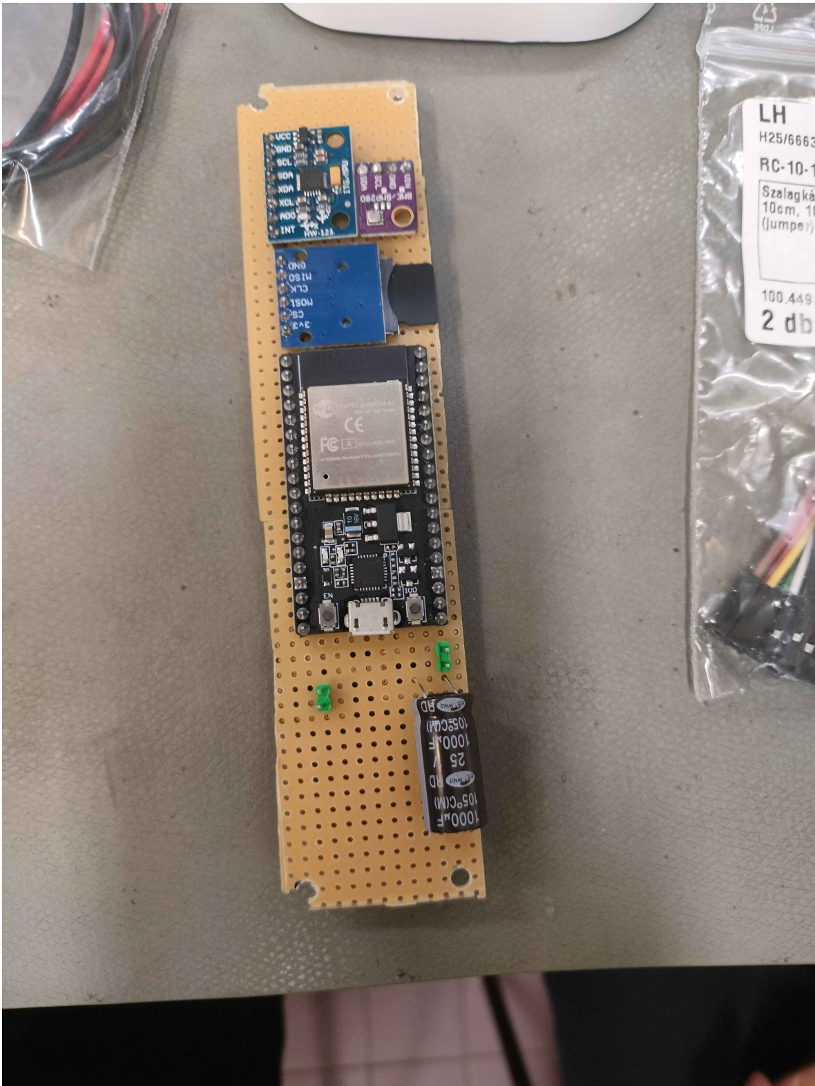
Figure 10: The panel's front side. Here, we can access the SD card and the ESP-32.
